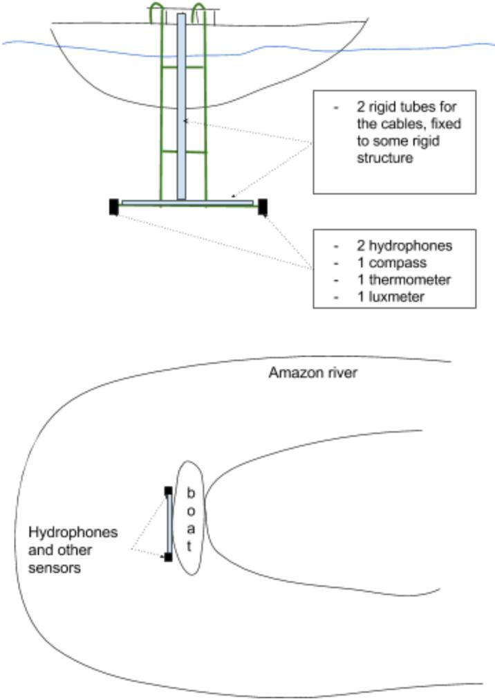
Figure 6 - System setting from the side (top) and from above (bottom) (scale is not respected).
