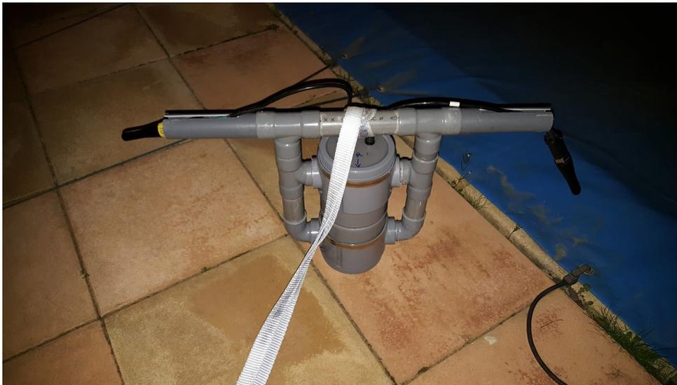
Figure 8 - Ultrasonic and environmental data acquisition system including 2 hydrophones (here not fixed) a luxmeter, a compass, a JASON board and batteries. The system can be powered during days by an external car battery.
