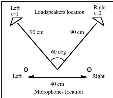
Figure 1: Set-up of the recording of ST-Numbers95
