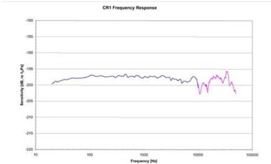
In addition a prototype Dolphin Recording System (DRS) was tested in the same Amazonian region in 2012. The system consisted of a Cetacean Research Technology CR 3 Hydrophone, a Reson preamp and an IOTech Personal Daq/3000 Series digital acquisition system. Recording sample rates were set at 400 or 500 kHz/second yielding recordings up to about 195 to 230 kHz. Below is the CR 3 Hydrophone response curve.
